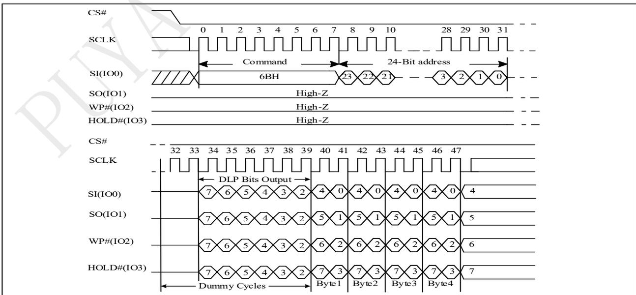
**Figure 10-23e 4IO Read with DLP bits output Sequence**
