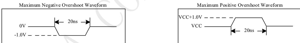
During DC conditions, input or I/O signals should remain equal to or between VSS and VCC. During voltage transitions, inputs or I/Os may negative overshoot to -1.0V or positive overshoot to VCC + 1.0 V, for periods up to 20 ns.
