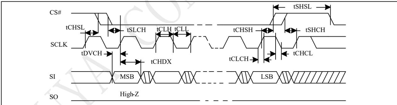
Figure 5-5 Output Timing
