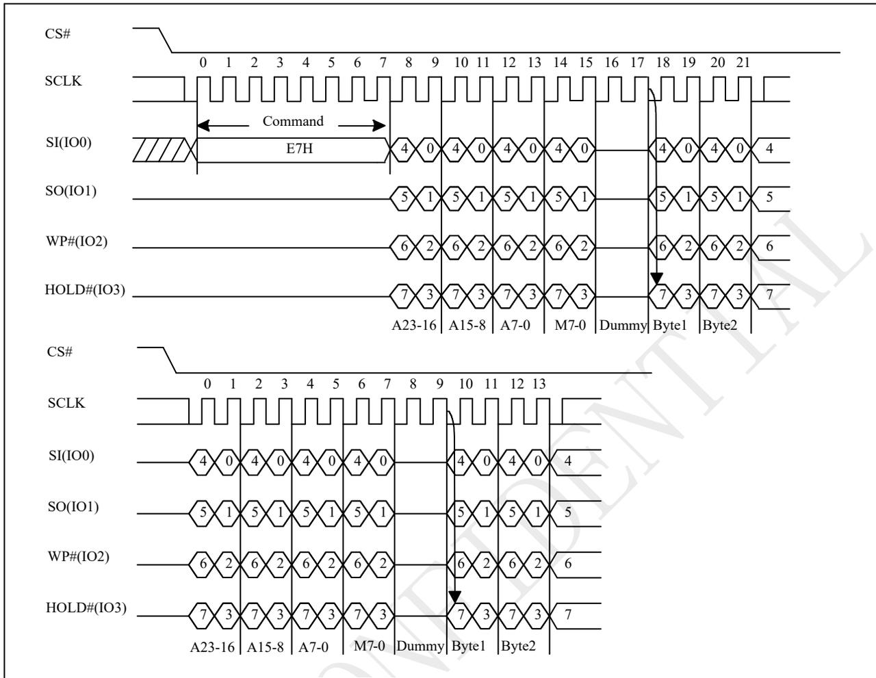
**4IO Word Read with “8/16/32/64-Byte Wrap Around “in Standard SPI mode**
