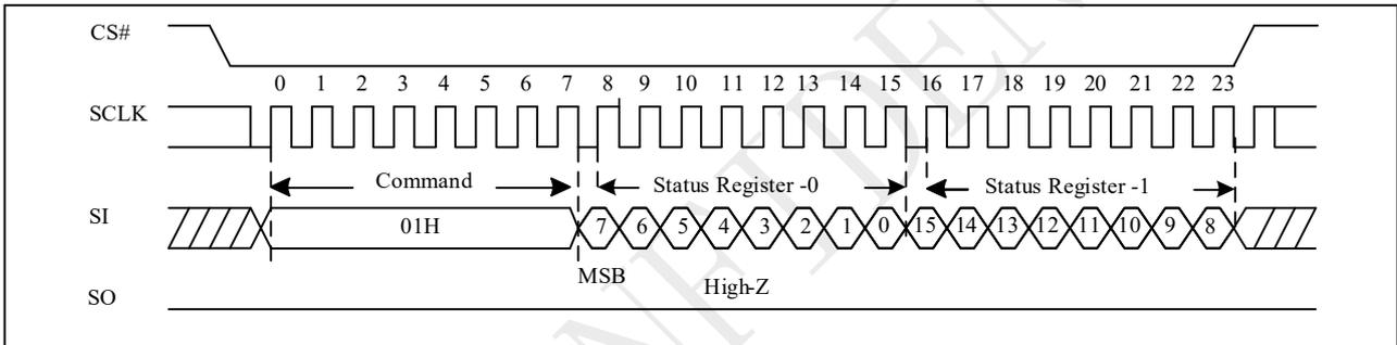
**Figure 10-7c Write Status Register (WRSR) Sequence (QPI)**
