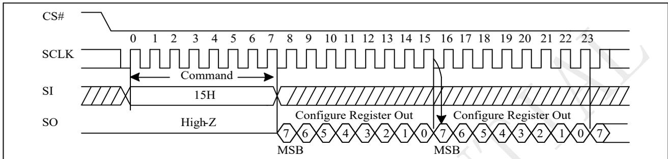
**Figure 10-6a Read Status Register (RDCR) Sequence (QPI)**
