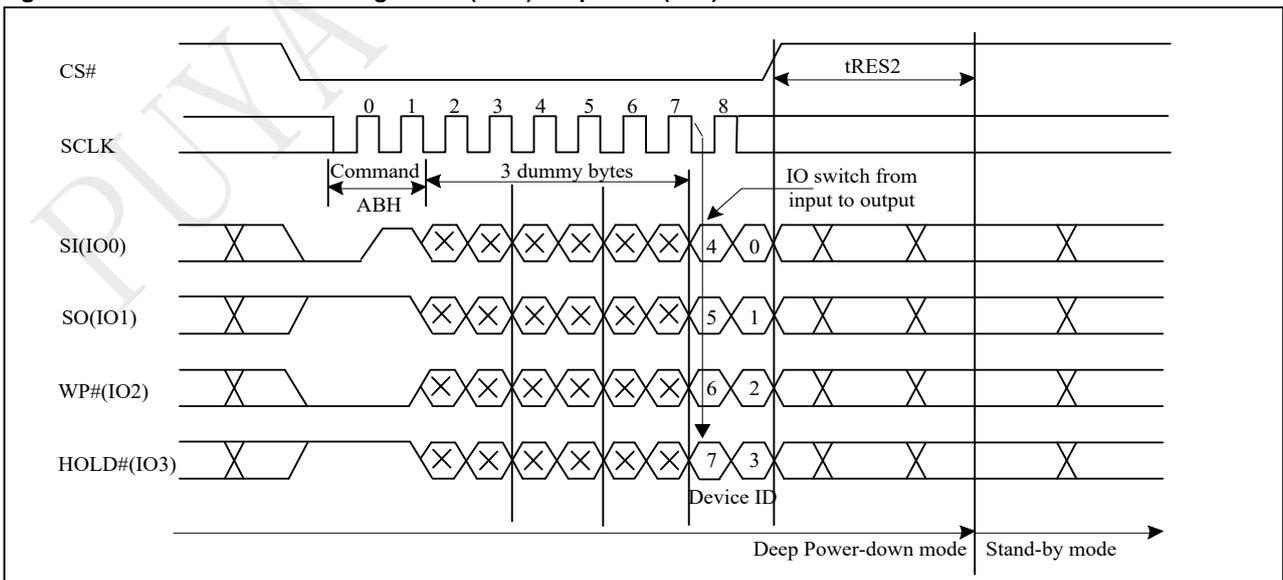
**Figure 10-36b Release from Deep Power-down (RDP) Sequence (Command ABh)**
