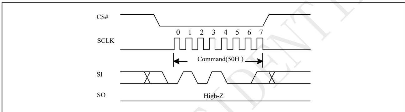
**Figure 10-4a Write Enable for Volatile Register Sequence (QPI)**
