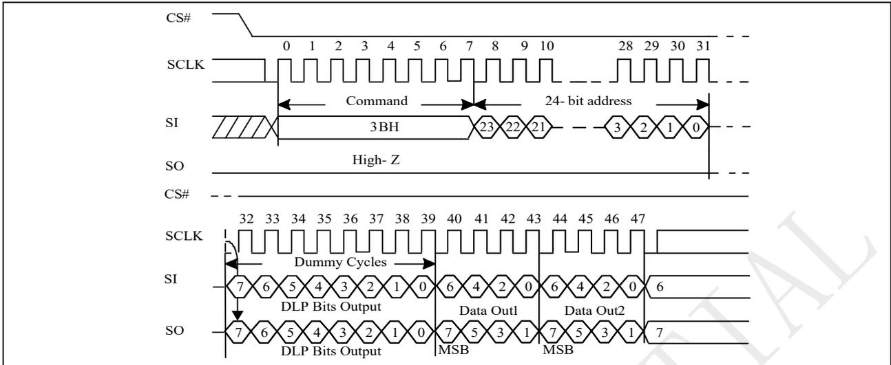
**Figure 10-23c 2IO Read with DLP bits output Sequence**
